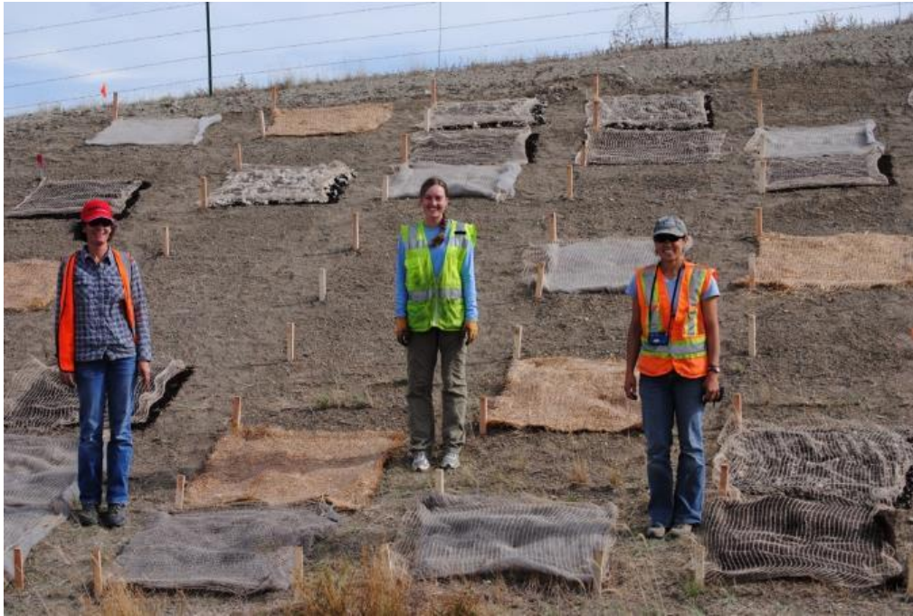
Figure 22: Replications of erosion control products along U.S. Highway 287, Three Forks, Montana, October 2014. Plot dimension is one meter square and all treatments are covered with mesh netting stapled in place.
