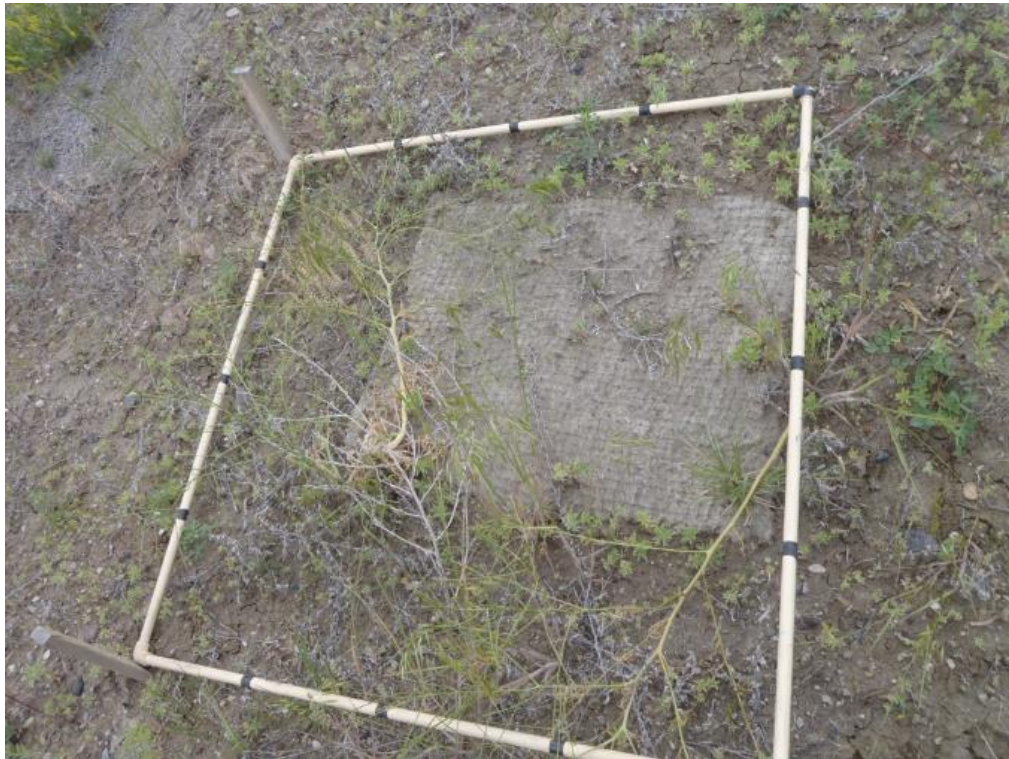
Figure 23: June 2016 field monitoring found shrinkage of a pure wool needle punched batt along U.S. Highway 287 near Three Forks, MT. The product initially covered the entire one square meter within the PVC frame
