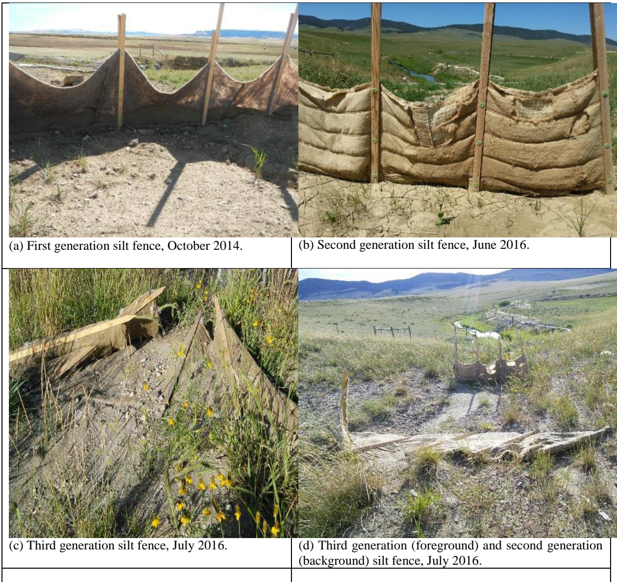
Figure 19: Photo monitoring the three generations of wool silt fence developed and tested in field trials along U.S. Highway 12, 2014 – 2016.
