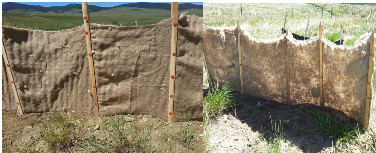
Figure 27: (a) Rolled silt fence constructed of two burlap layers sewn together with cut wool pieces as filler. (b) Backlit burlap and wool silt fence shows the lack of consistency in the distribution of the wool pieces in the center layer of the fence.
