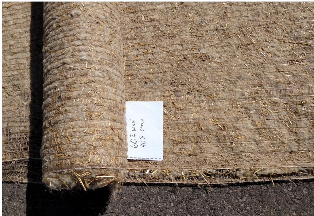
Figure 24: Example of wool combined with straw as fill between two biodegradable net layers in a rolled erosion control blanket.
