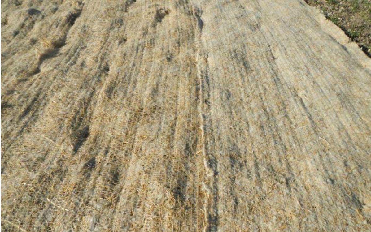
Figure 7: Demonstration of two erosion control blankets using different ratios of wool and straw produced by Ero-Guard.
