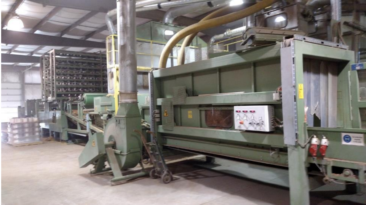
Figure 25: Equipment that manufactures rolled ECBs, Ero-Guard, Mapleton, MN.
