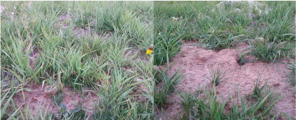
Figure 10: Seedlings are able to penetrate the 68 \text{ g/m}^2 and 136 \text{ g/m}^2 carded wool batting (left), but had difficulty penetrating the 203 \text{ g/m}^2 and 271 \text{ g/m}^2 carded wool batting (right).
