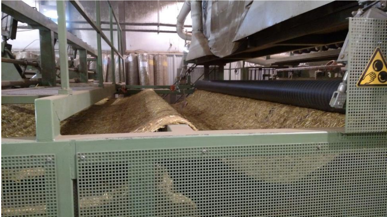
Figure 26: Close-up of a straw and jute net ECB manufacturing at Ero-Guard, Mapleton, MN.
