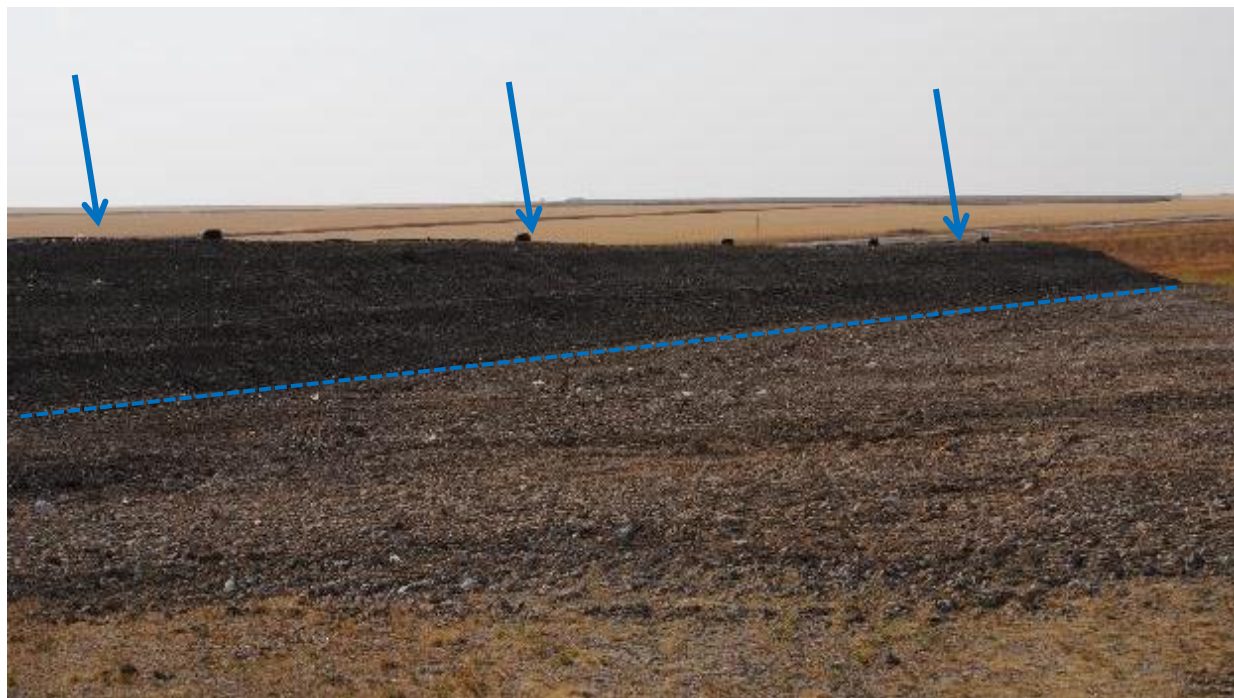
Figure 17: Test slope (2H:1V) constructed at Transcend, a WTI-MSU experimental station in Lewistown, MT.
