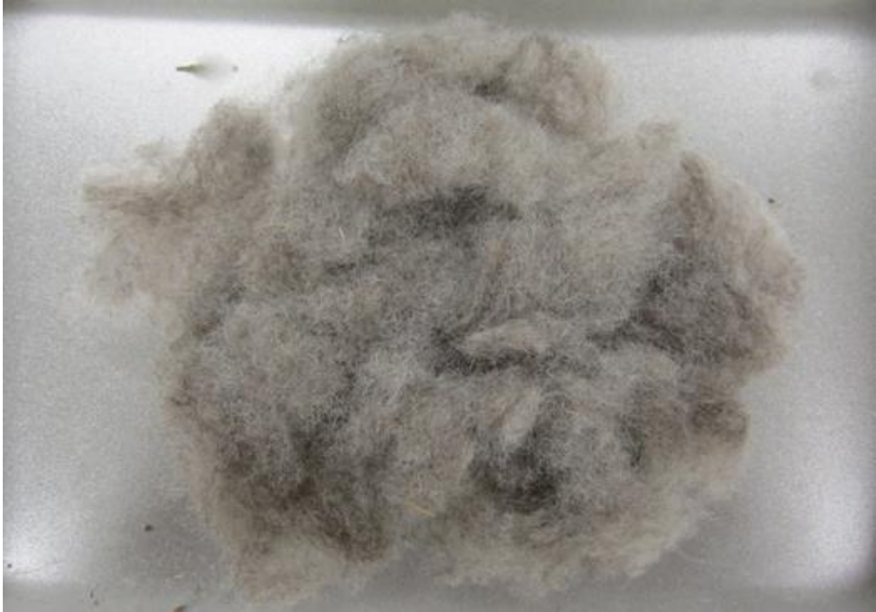
Figure 6: Washed, scoured and shredded wool sample from Brookside Woolen Mill.
