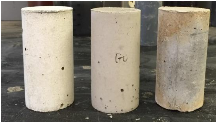
Cement mortar (left); GO-modified fly ash mortar (middle); fly ash mortar (right)
